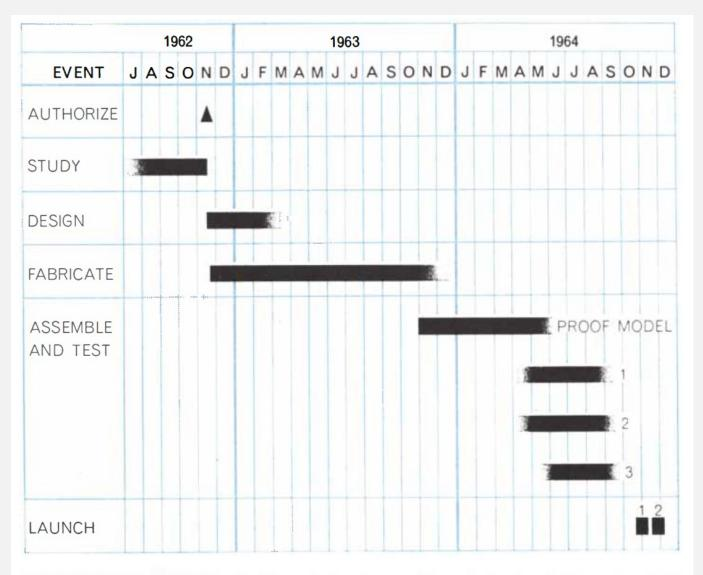
MARINER SCHEDULE for the Mars mission began with authorization in November, 1962, based on prior studies. The chart shows how it was necessary to compress design, fabrication and testing to have three flight-qualified spacecraft ready for launching by November, 1964.
